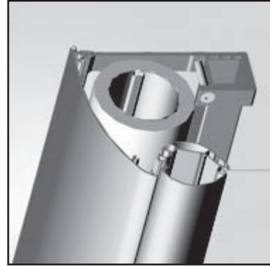
The fabric is protected with an aluminium powder coated extruded cover.
